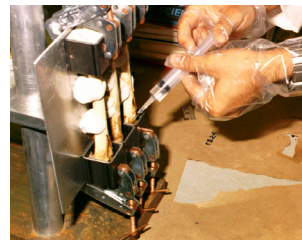
A potting compound is poured into sockets. After it is cured, samples are flipped over and other end is bonded
